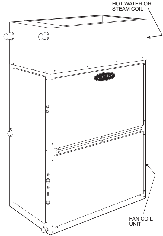
40RU WITH HOT WATER OR STEAM COIL
