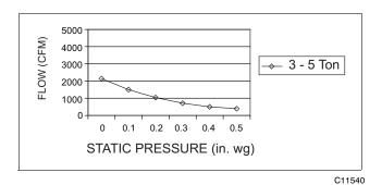
Fig. 7 - Vertical Power Exhaust Performance
