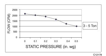
Fig. 10 - Horizontal Power Exhaust Performance
