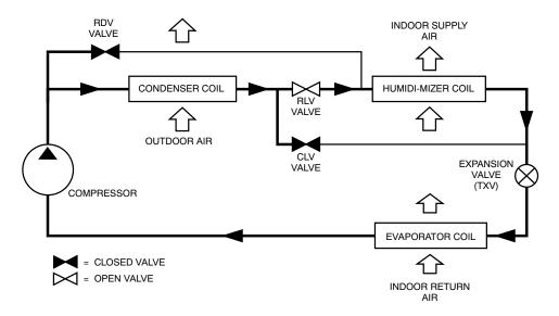
Fig. 14 - 48LC 04-06 Subcooling Mode (Reheat 1) - Humidi-MiZer System
