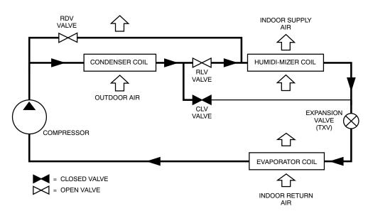
Fig. 15 - 48LC 04-06 Hot Gas Reheat Mode (Reheat2) - Humidi-MiZer System
