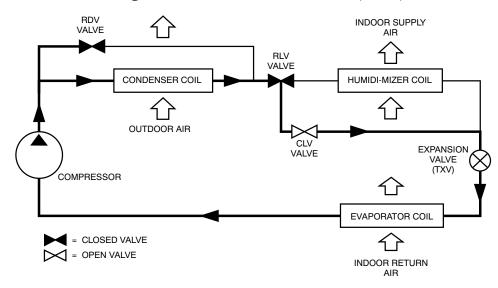
Fig. 13 - 48LC 04-06 Normal Cooling Mode - Humidi-MiZer System
