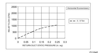
Fig. 8 - Barometric Relief Flow - Horizontal 3 - 5 Ton
