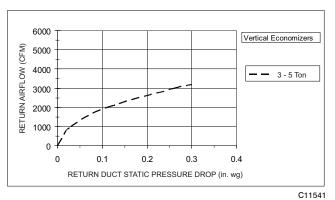
Fig. 6 - Return Air Pressure Drop-Vertical 3 - 5 Ton
