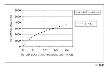
Fig. 9 - Return Air Pressure Drop - Horizontal 3 - 5 Ton
