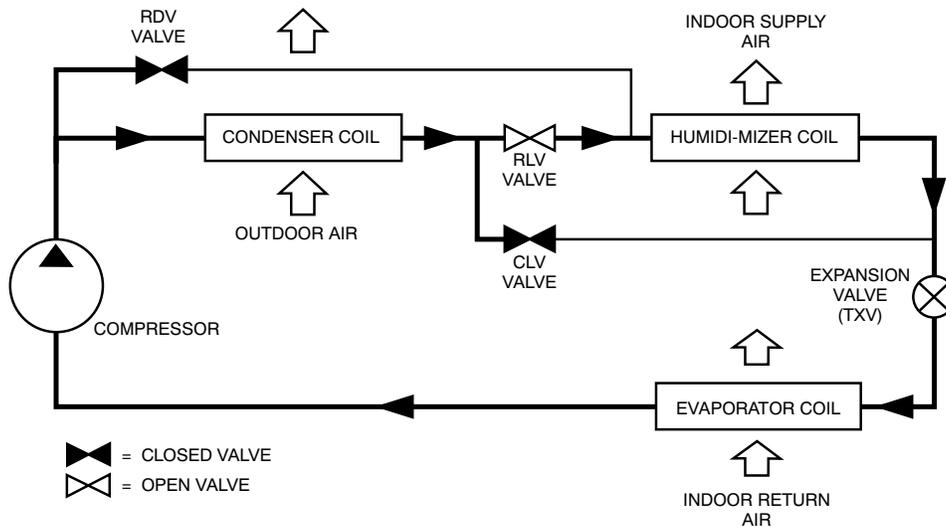
**Fig. 14 - 48LC 04-06 Subcooling Mode (Reheat 1) - Humidi-MiZer System**
