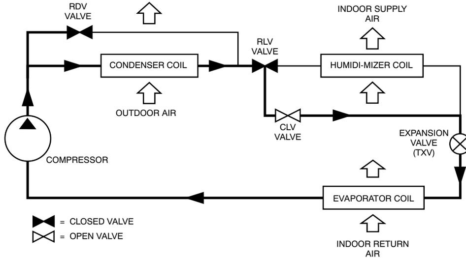
**Fig. 13 - 48LC 04-06 Normal Cooling Mode - Humidi-MiZer System**
